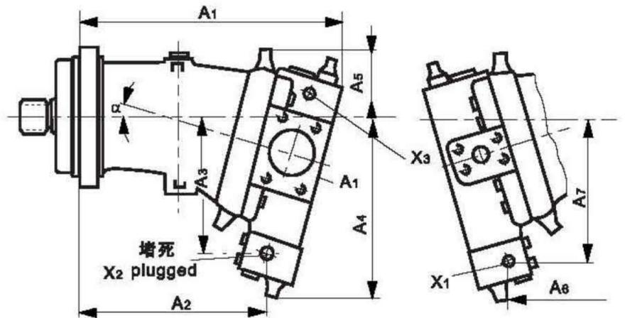
A<sub>1</sub> 和 X<sub>3</sub> 仅用于带压力切断 A<sub>1</sub> and X<sub>3</sub> with pressure cut-off only
