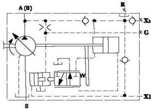
辅助元件: 压力切断 Auxiliary Equipment: Pressure Cut-Off
