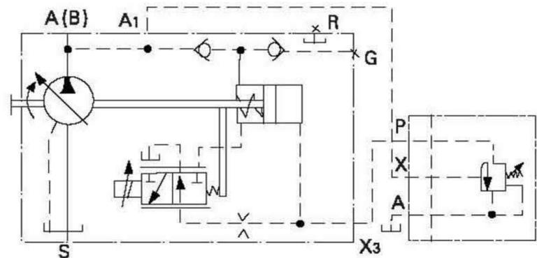
EP 带压力切断的电控比例变量 Electric Pro.Control with Pressure cut-off 接口 Connections
